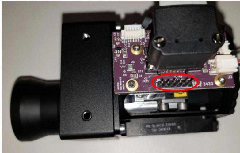
*Figure 7 Serial Connection*
