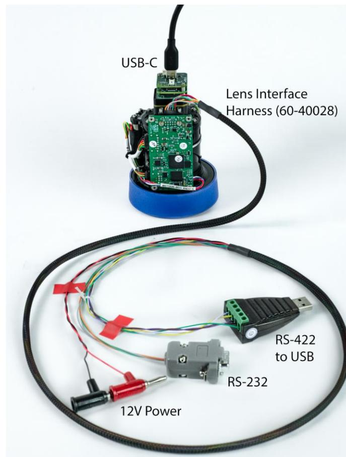
**Figure 1: Lens Interface Harness (60-40028) and USB-C Cable**
