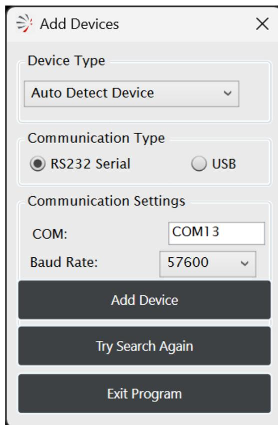
**Figure 5: CCS Manually Add Device**
