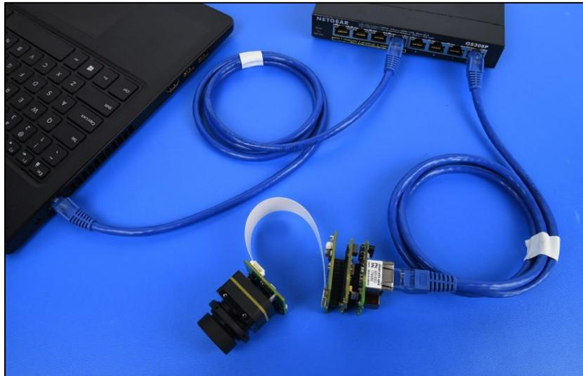
*Figure 2 Ethernet Connection with PoE Switch*
