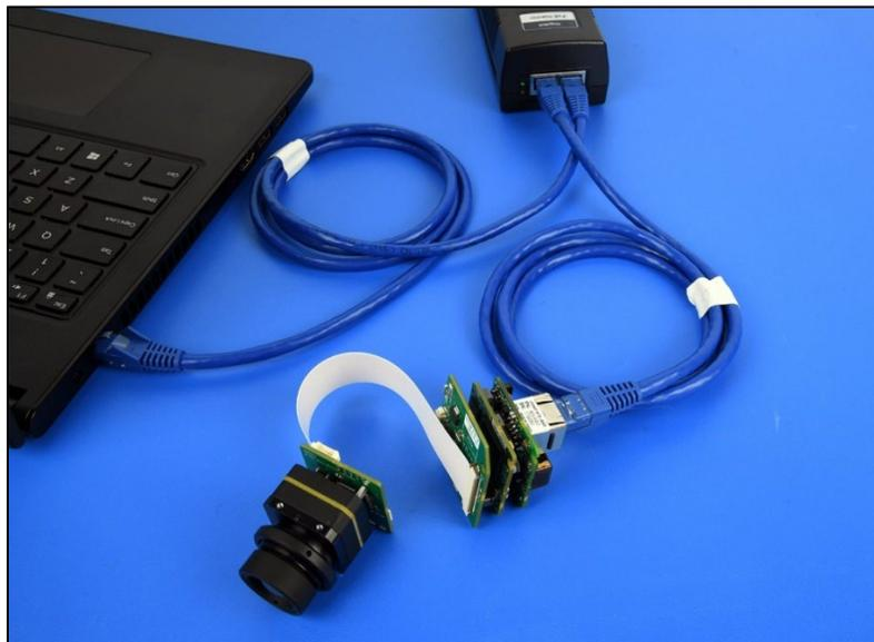
*Figure 1 Ethernet Connection with PoE Injector*
