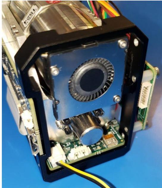
*Figure 3: Connect the Power*
