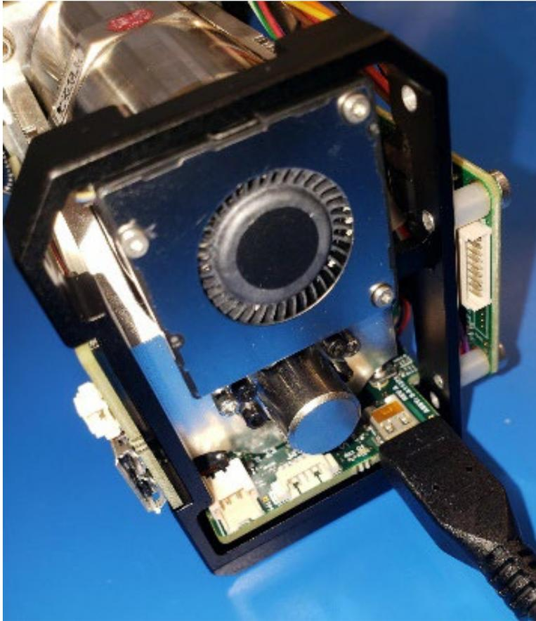
*Figure 2: Connect the HDMI*
