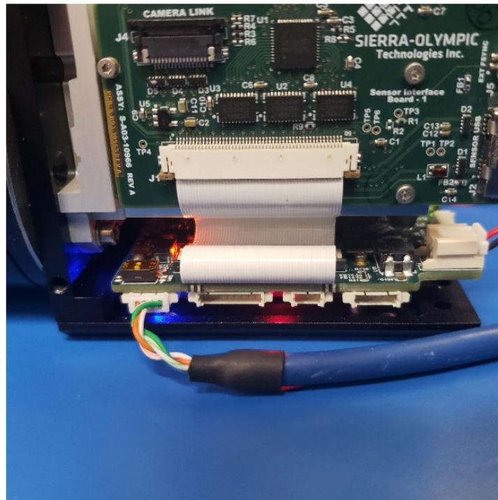
*Figure 1: Connect the Ethernet*
